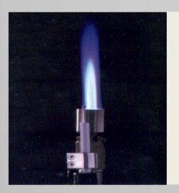
Flame treatment air/ propane (22:1); variation of exposure time, burner capacity, and flame distance additionally: flame treatments under industrial conditions in a paint line
