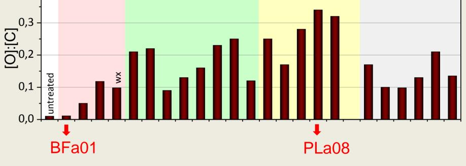
High fluctuations in the oxygen content of the outermost surface region
