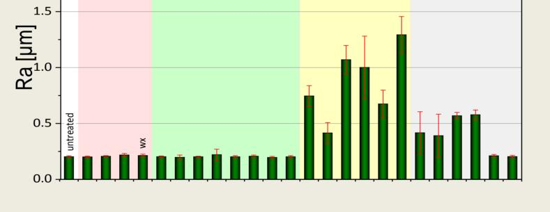
Plasma jet treatment: surface roughness and heterogeneity were dramatically increased depending on the treatment parameters
