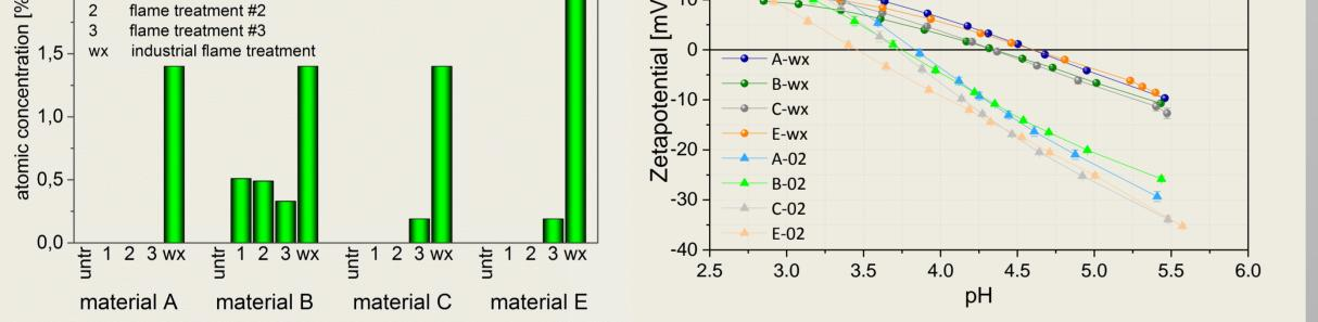
TPO surfaces treated in a paint line contained higher amounts of nitrogen resulting in a change of the acid-base properties
