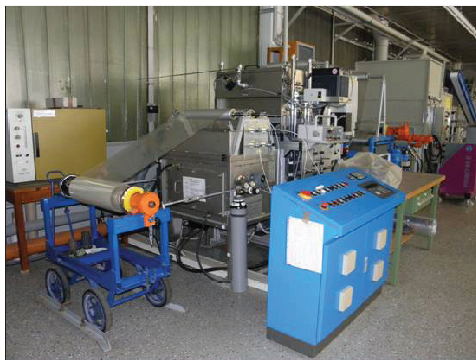
Figure 2: Pilot plant for oxo-fluorination
