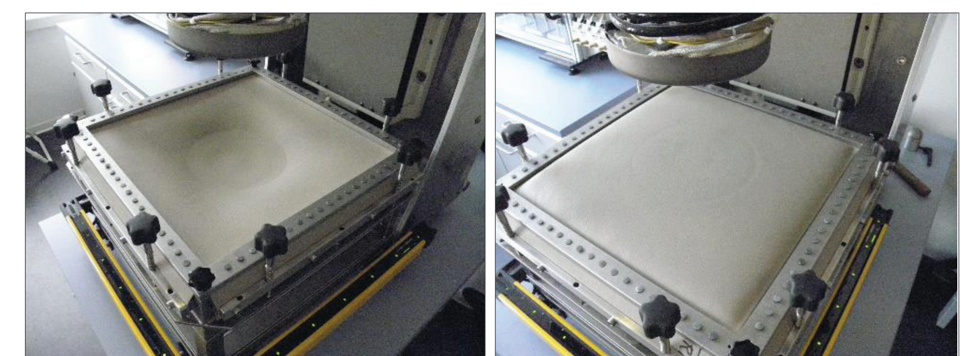
Figure 5: Images of clamp-fixed leather samples after five test cycles without (left) and with PUR foam cushion (right).
