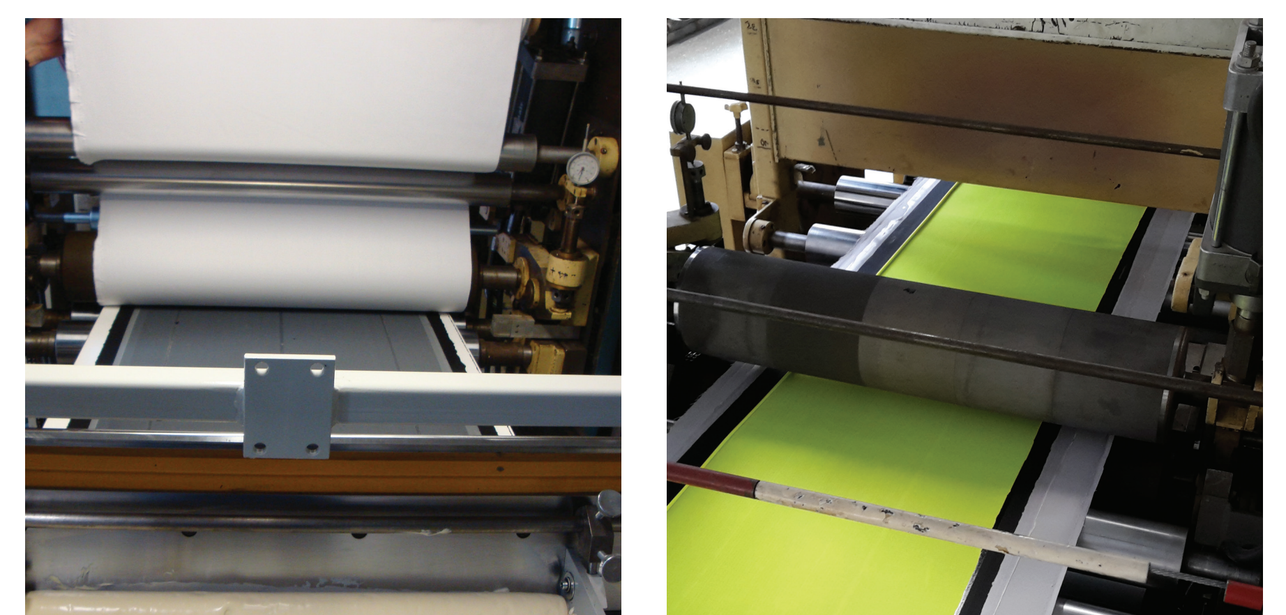
Fig. 4: application of adhesive coat and textile lamination
