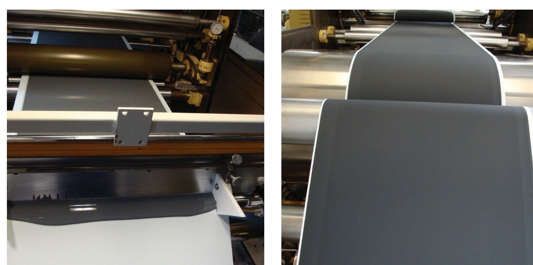
Fig. 2: blade coating facilities in technical scale
