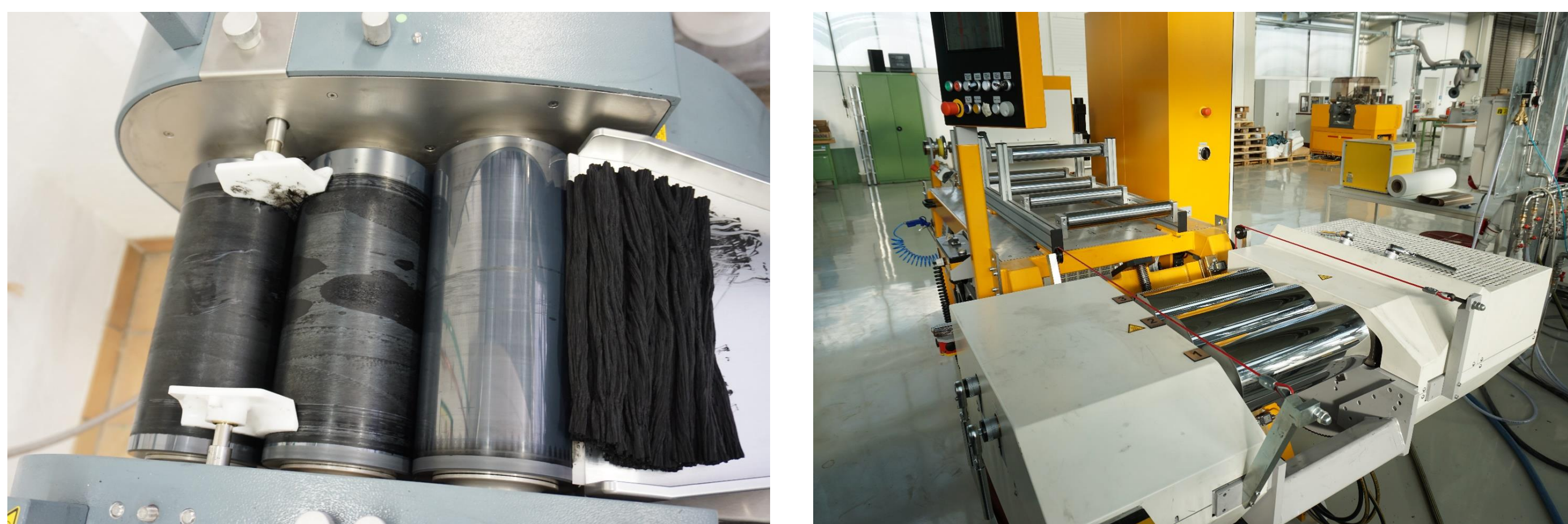
Fig 2: left picture - incorporation of MWCNTs in a silicone matrix on a 3-roll mill right picture - processing of silicone MWCNT composite masses on the 3-roll calender
