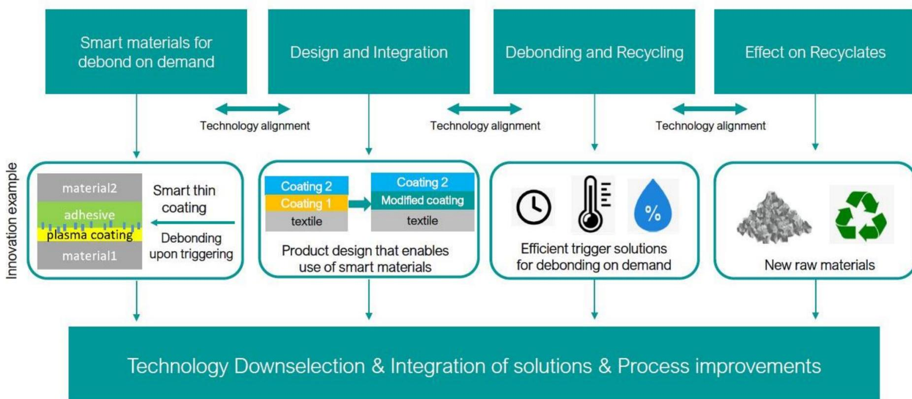
Figure 1: An integrated approach for Debonding on Demand
